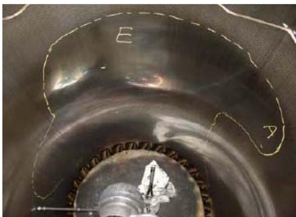
Fig.4 、 Polish on cylinder liner.
