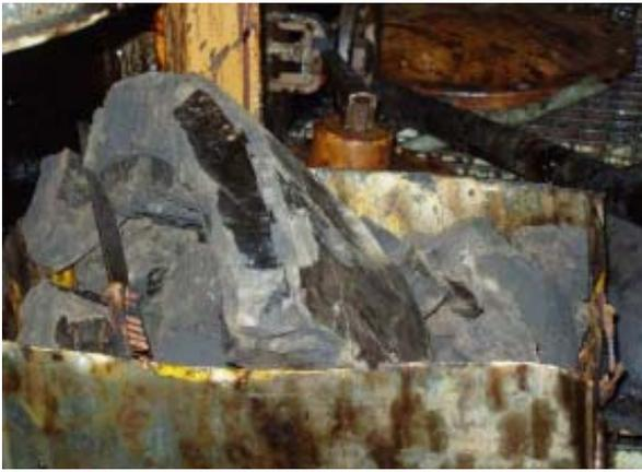
Fig 1 、 Hard Sludge from Separator
